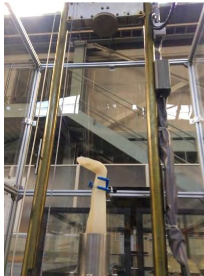
Figure 3. A scene of falling-weight impact test.
