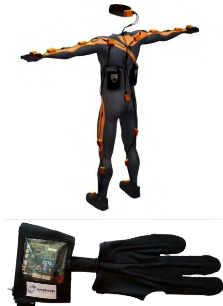
Figure 1. Wearable sensors used in the experiment: (a) Xsens MVN suit; (b) e-glove from Emphasis Telematics.
