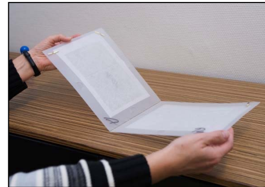
Electrostatic dust collector (EDC)
